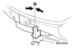
On full-pivot system models, tighten the steering friction adjuster by turning it clockwise to prevent the motor from turning freely.
